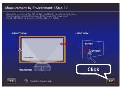
Position the sensor at approximately 30cm from the edge of the projected image with it in contact with the screen, and make sure the LED is facing the projector.
