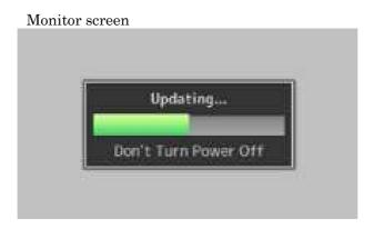
(3) After updating is complete, "Complete" appears in the output screen. Power LED: blinking "Blue"
