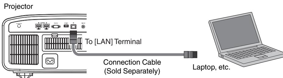
Connect the projector to a PC via LAN cable.
